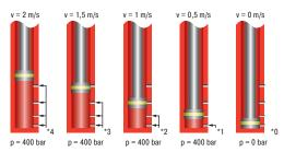
\* The load velocity reduces continuously as you travel through the stroke due to the reduction in the number of metering orifices (\*) in action. The internal pressure remains essentially constant and thus the Force vs. stroke curve remains linear.
