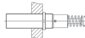
Tightening torque: 80 Nm
